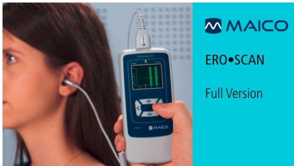
Figure 3: Concept image of the MAICO OAE device used by the midwives, presented during the co-design interview. The screen displays two bars representing the frequencies that have been passed during the test.
